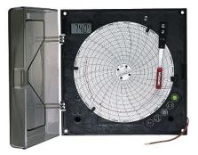
**Temperature Recorder** Easily Installed into the Freezer control Panel.
